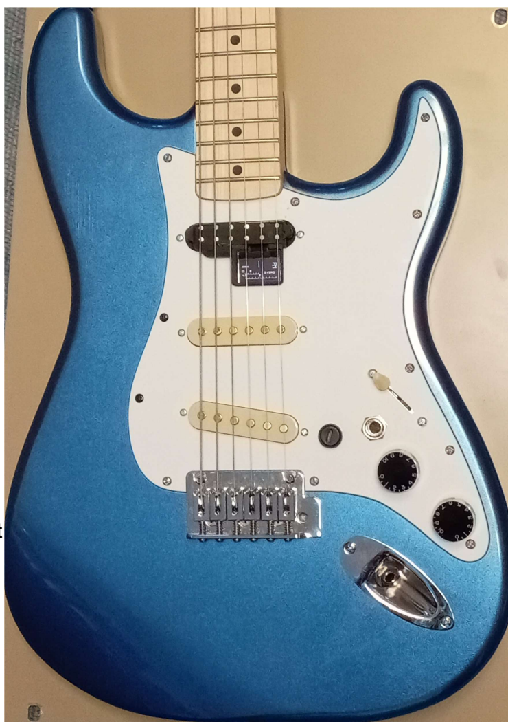
Figure 2: The pickguard modified for use with the \mu PGV in the case of the single coil -sized variant. Additional vocal microphone mini XLR connector and a USB-C charger jack are needed. The hole of the removed second tone knob is used for the USB-C charger jack. The volume and the other passive pickup tone knobs stay at their normal positions.
