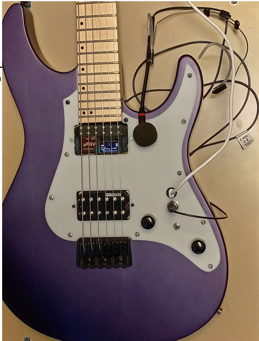
Figure 3: The pickguard modified for use with the humbucker -sized variant. The vocal microphone and the USB-C charger are also shown connected. The selector switch now has only two positions, either for the \mu PGV or for the remaining bridge pickup.
